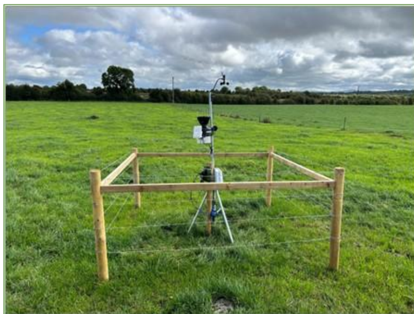
Plate 2.2 - Weather station installed near T1.
