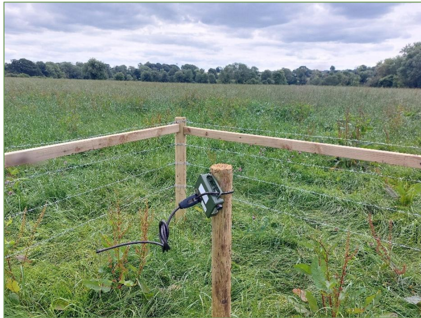
Plate 2.1 – Example of Song Meter Mini Bat Ultrasonic full-spectrum detector deployed at a proposed Turbine location.
